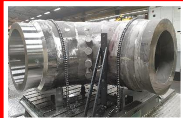
Primary Circuit Elbow (~8T)
